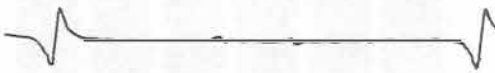
Fig.1[B]. ESR spectra of DMPO spin adducts formed in the Fenton reaction without (A) or with NPH4 of 0.5mM (B) and 1.0mM (C). Each spectrum was obtained at 60 sec after adding hydroperoxide. Signals appearing both at high and low field are due to Mn (II) installed in the cavity as a reference. the main species present is DMPO-OH.
