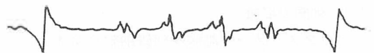
Fig.1[A]. ESR spectra of DMPO spin adducts formed in a hypoxanthine/xanthine oxidase (HPX/XOD) system without (A) or with NPH4 of 0.5mM (B) and 1.0mM (C).
